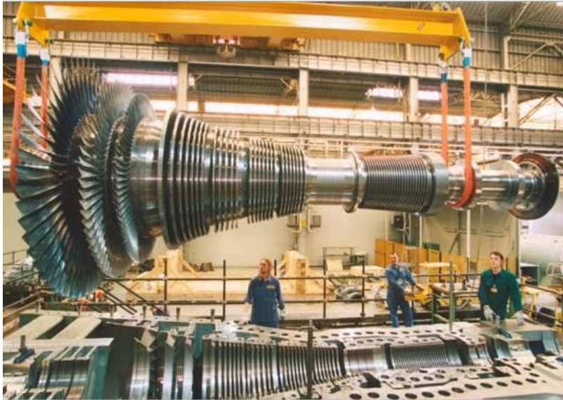
56 MW GE steam turbine with 400 mm diameter tilting pad journal bearings (Courtesy of GE)
